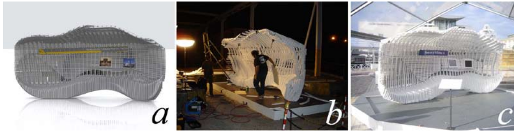
Figure 1 CNC Cut Bus Stop starting with the initial shape in CAD (a), CNC cut components as- sembled by hand (b) and the final artifact (c)
